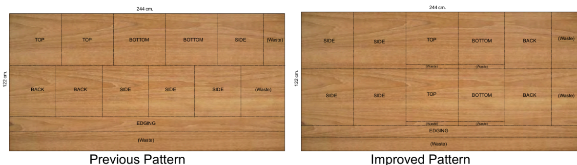
Figure 7: (Left) Plywood Cutting Pattern - Before Improvement; (Right) Plywood Cutting Pattern - After Improvement
